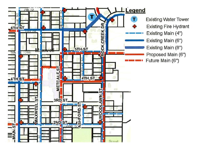
"O"- 6" Water Line and Main Line Valve Replacement Plan
