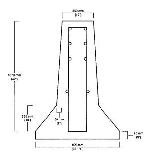
Using 12' long Jersey concrete highway barriers to establish side walls and one end wall to retain sand and salt mixture.
